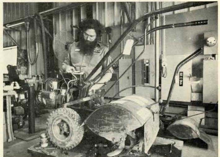
Service after-the-sale is still the most important product. No matter how used or abused, every Tiller can be completely rebuilt for one-half the price of a new one.
