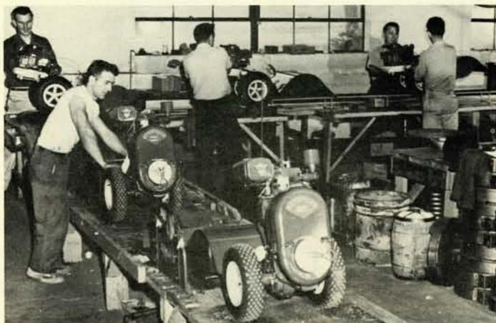
Improvements to the machine were accompanied by improvements in the manufacturing process. By the mid-fifties, the ROTOTILLER factory was capable of turning out a new tiller every 6½ minutes. In the photo above, Joe Zakrzewski checks final assembly. Four members in two generations of the Zakrzewski family are still turning out Tillers in Troy.
