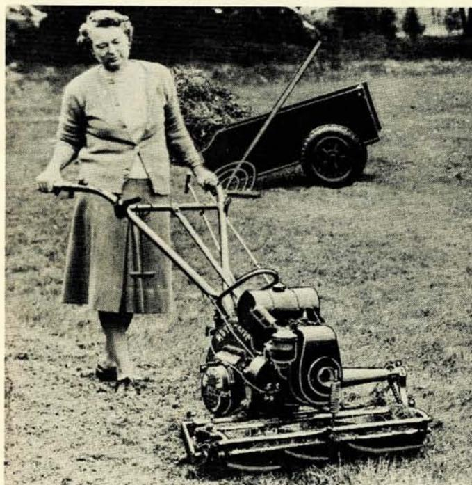
A *Roto-Ette* lock-reel mower attachment had a "floating head" feature which let the user mow over rough or uneven terrain without skips or "scalping".
