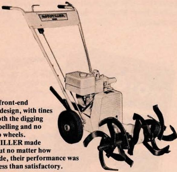
The original design of all rotary tillers had the tilling unit in the rear of the machine and powered wheels to propel it forward. In 1936, a machine which was just the opposite was designed. The front-end tiller had no power to its wheels and depended upon the action of its front-mounted tines to pull the machine along the ground.
