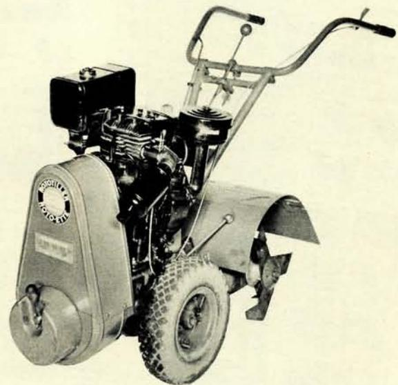
Only a very few of the Model 5 tillers were made in 1956 and, unfortunately, none remain in original condition now. They were unique in that the tine and hood assembly was removable for the attachment of other powered accessories at the rear of the machine.
