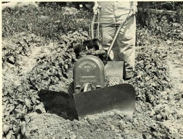
Another “Lightning Change” attachment to the Model 2 Rototiller was this earth grader/snow plow.
